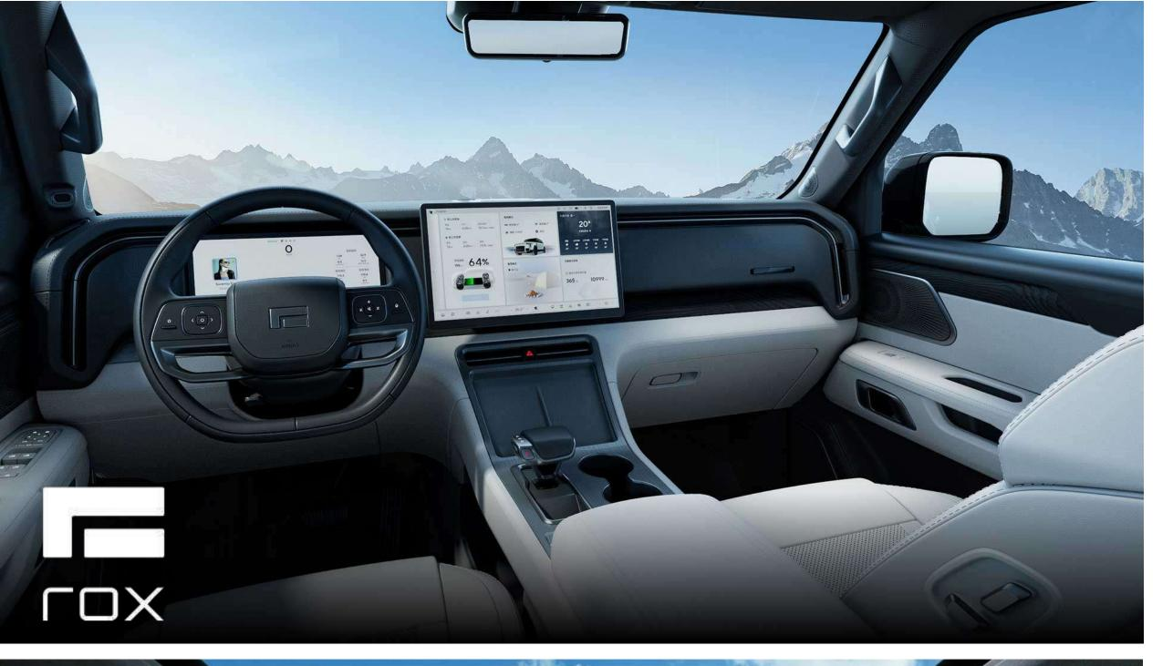
Standard configuration is a 12.3-inch instrument screen, a 15.7-inch 3K ultra-clear central control screen and 9-inch rearview mirror.
